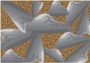
Conceptual diagram of structural soil (Bassuk, 2007)
